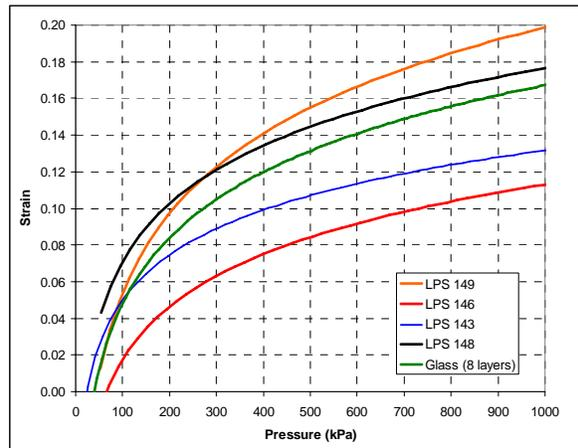
Fig. 4 A comparison of the compaction characteristics for the glass-aluminum hybrid preforms and glass fabric.
