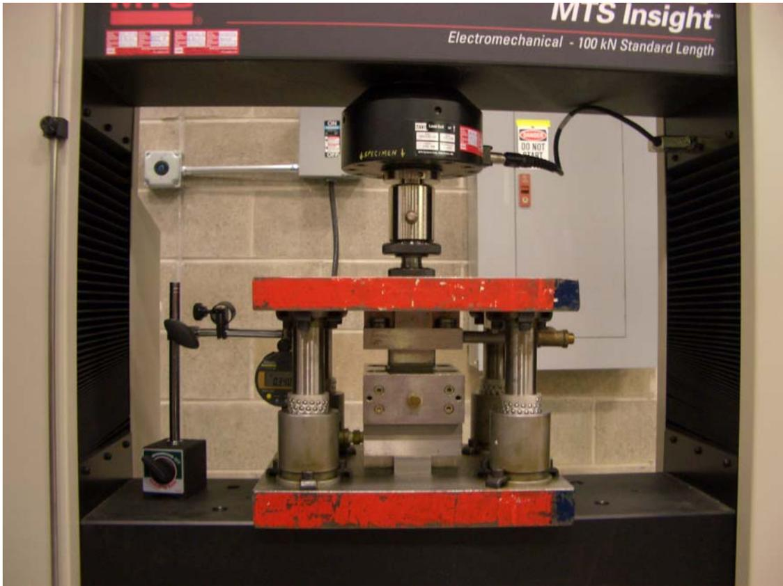
Fig. 2 Compaction test fixture.
