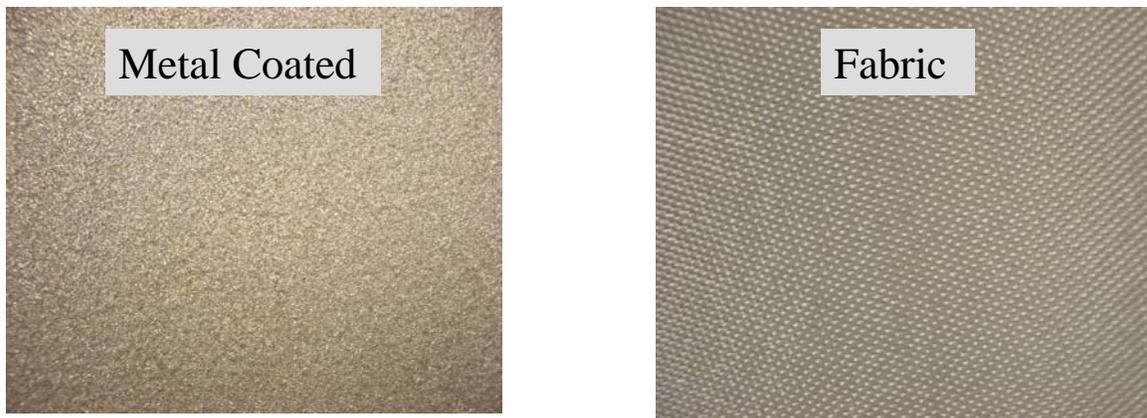
Fig. 1 S2-glass fiber, 8HS woven fabric single side coated with an aluminum alloy at a deposition of  $0.37 \text{ g/in}^2$ .
